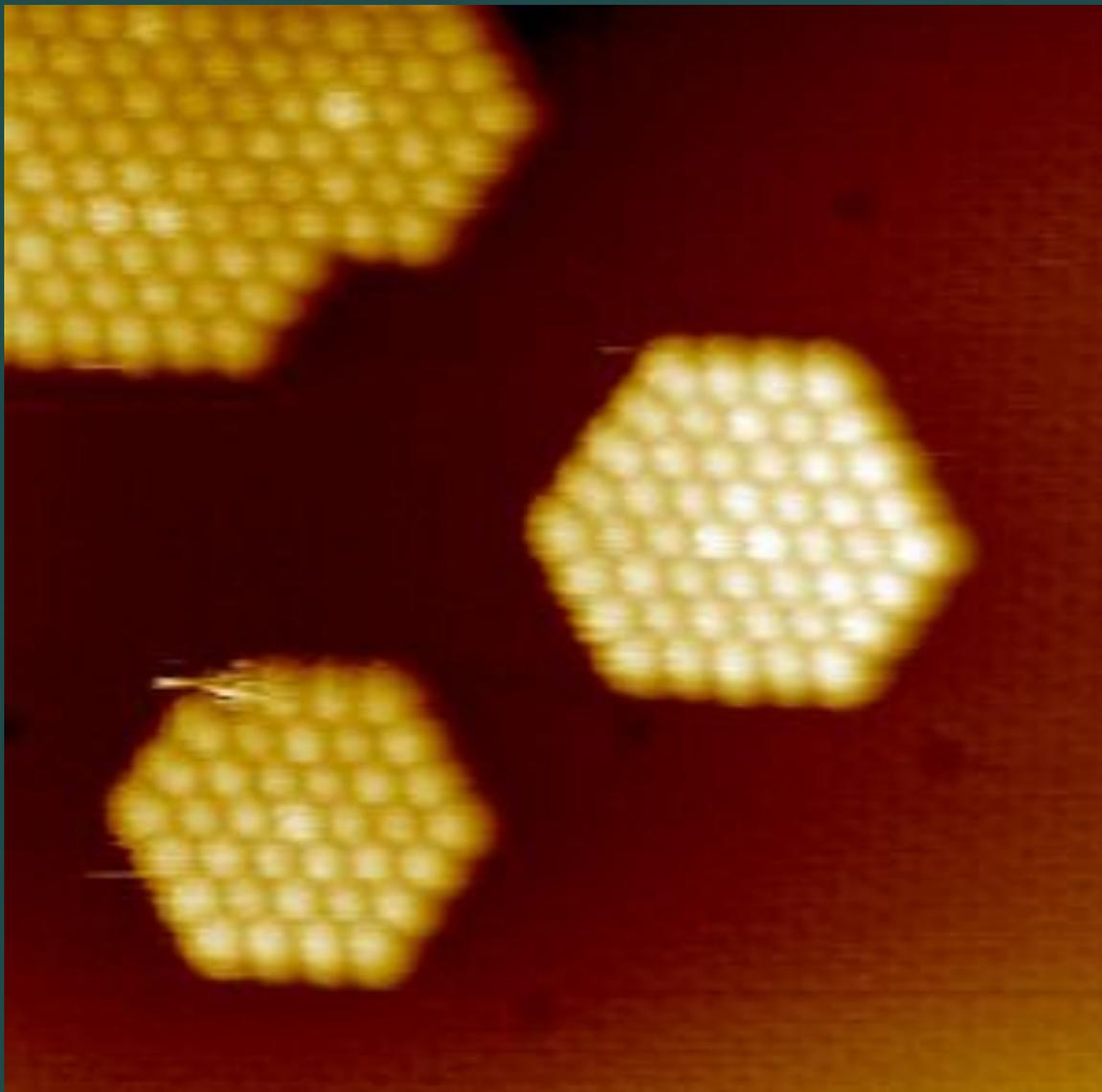
Snapshots illustrating the dynamic process of  $C_{60}$  island ripening towards the more stable forms.
