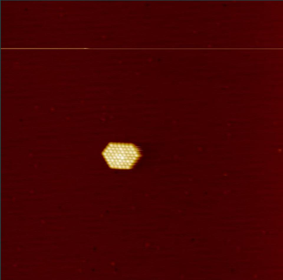
When C<sub>60</sub> flux is switched on, the 56-mer starts to grow through the successive formation of the high-generation magic islands. This growth in the island size exhibits a stepwise dependence versus C<sub>60</sub> deposition time.
